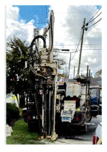
is completed, each borehole will be filled in and the surface will be restored to its original material (e.g., grass, gravel, asphalt, concrete). The public should expect a high level of noise when drilling (from 8 am to 5 pm on weekdays only) and the presence of trucks with auxiliary equipment during the sampling.
